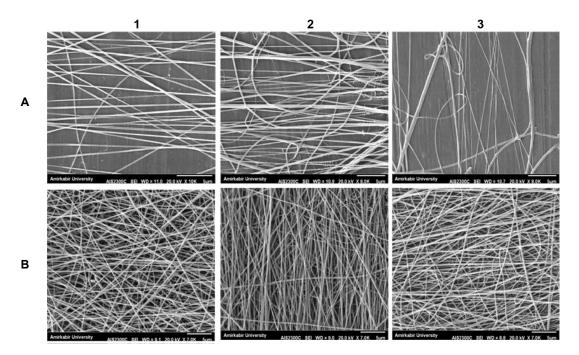
**Fig.2:** Scaffold homogeneity analysis by scanning electron microscopy (SEM) micrographs of the aligned polycaprolactone (PCL)/gelatine (70:30) with different electrospinning parameters (Table 1) for the A1, A2, A3, B1, B2 and B3 samples.
