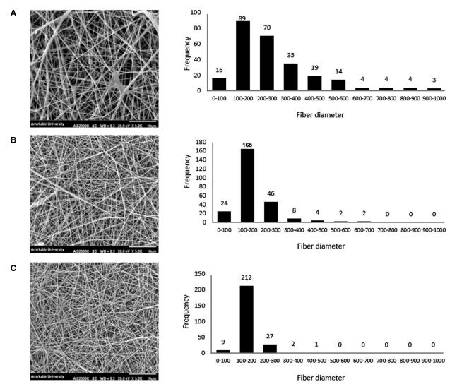
Fig.3: Scanning electron microscopy (SEM) micrographs and fibre diameter frequency of the random: A. polycaprolactone (PCL)/gelatine (60:40), B. PCL/ gelatine (70:30), and C. PCL/gelatine (80:20).
